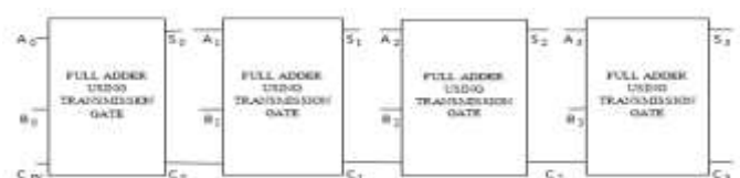
Fig. 1 Block diagram of 4-bit Full Adder using transmission gate.
