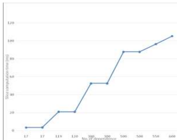
Fig. 6. Graph showing No. of Dep.Vs Dynamic Slice Computation Time in Milli Sec.
