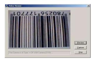
Fig. 10 Decoding barcode area displaying the resulted barcode number
