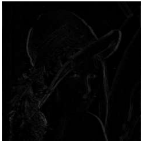
Fig. 3 Edge detection by the F^0 -transform - Image edge function E_r (10 pixels covered by one basic function).
