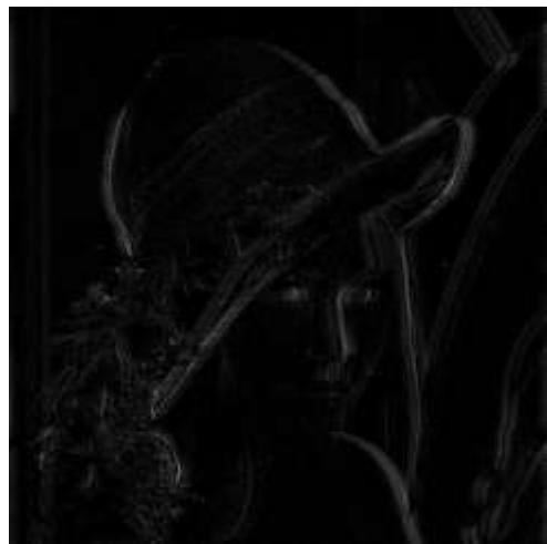
Fig. 4 Edge detection by the F^0 -transform - Image edge function E_r (20 pixels covered by one basic function).
