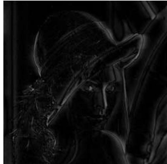
Fig. 5 Edge detection by the F^0 -transform - Image edge function E_r (50 pixels covered by one basic function).
