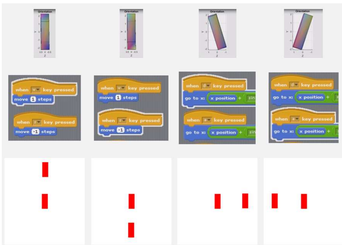
Fig. 10 Movement of the PC game's character according to the movement of the smartphone device
