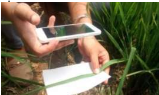
Fig 1 Proposed mobile device-based rice leaf analyzer structure for nitrogen estimation
