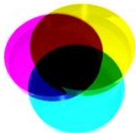
Fig. 4 Layers of simulated glass show how semi-transparent layers of color combine on paper into spectrum of CMY colors.
