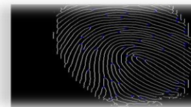
K. Final extracted Minutiae after applying the windowing technique
