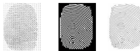
Fig(3) a. Orientation Field, b. Enhanced Image c. Thinned Image.
