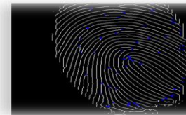
J. Minutiae obtained after deleting spurious minutiae at the borders
