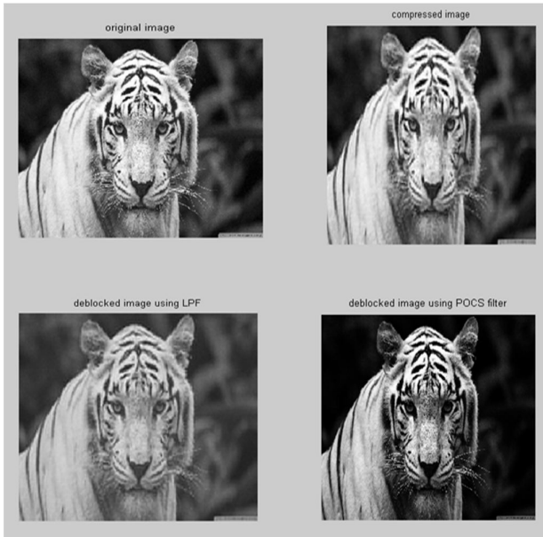
Fig. 3: Reconstructed images of Tiger image with quantization step 80. No filter (PSNR = 29:38dB, PSNR-B = 26:52dB, SSIM = 0:7700). POCS de-blocking filter (PSNR = 29:31dB, PSNR-B = 29:31dB, SSIM = 0:7926).
