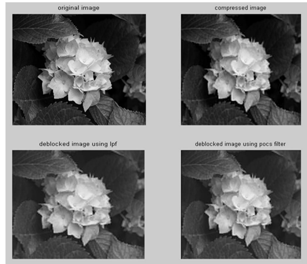
Fig. 5: Reconstructed images of Flower image with quantization step 80. No filter (PSNR = 29:88 dB, PSNR-B = 27:48 dB, SSIM = 0:7680). POCS de-blocking filter (PSNR = 29:91 dB, PSNR-B = 29:91 dB, SSIM = 0:8053).
